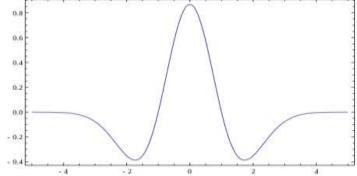
is the negative normalized second derivative of a Gaussian function,
