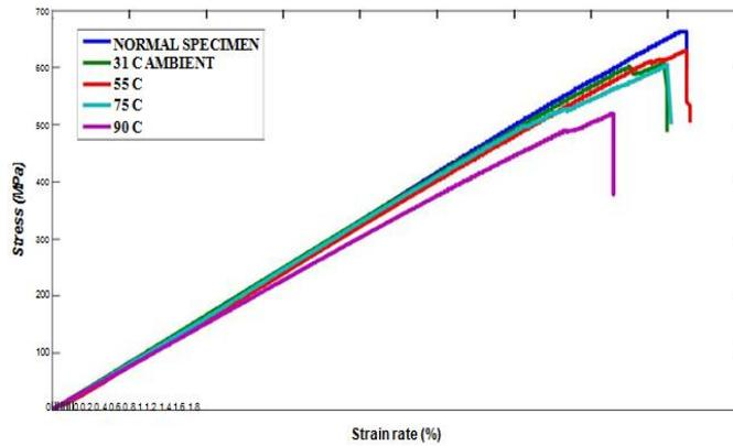
*Fig.4.4.a. Stress Vs Strain for Zero ply specimens*
