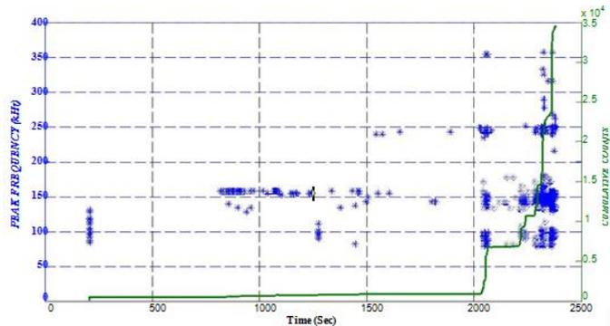
*Fig.4.5.n. Time vs. Peak frequency and cumulative counts-Zero Ply specimen*
