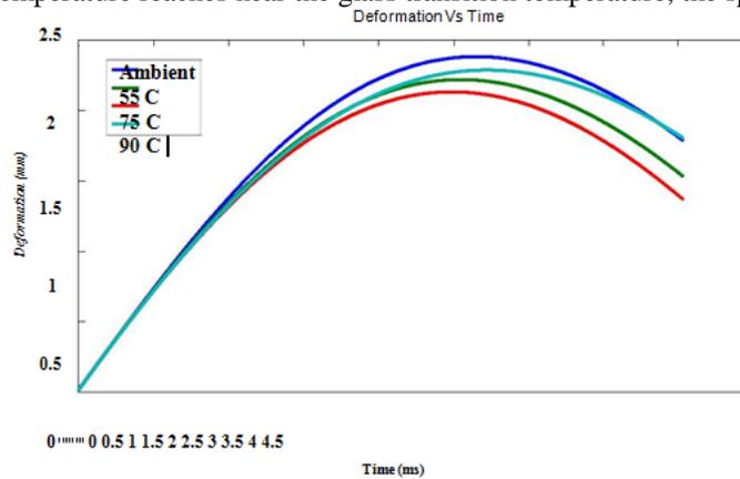
*Fig.4.3.d. Deformation vs. time for Cross ply specimens*
