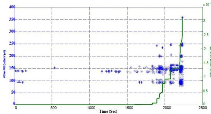
Fig.4.5.j. Time vs. Peak frequency and cumulative counts-Zero Ply specimen
