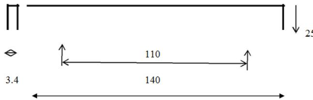
**Fig.3.c. Flexural Specimen (All dimensions are in mm)**
