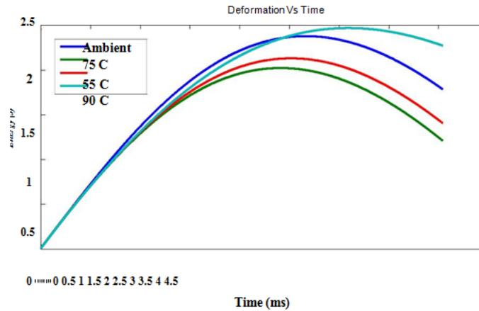
*Fig.4.3.c. Deformation vs. time for Zero ply specimens*
