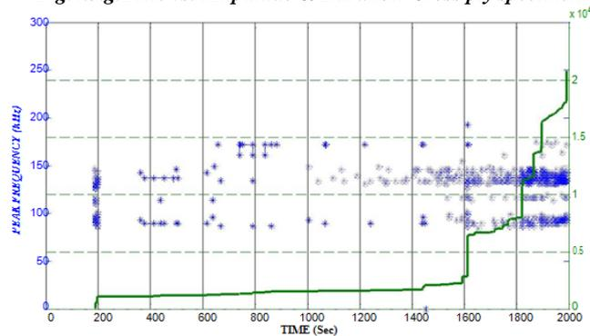
**Fig.4.5.h. Time vs. Peak frequency and cumulative counts-Cross Ply specimen**
