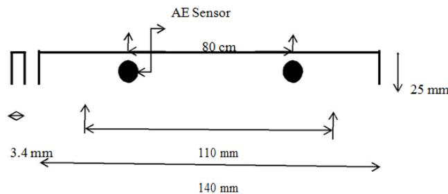
*Fig.3.i. Flexural Specimen with sensor position*
