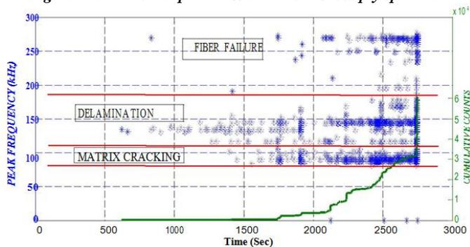
**Fig.4.5.d. Time vs. Peak Frequency & Cumulative Counts -Cross ply specimen**
