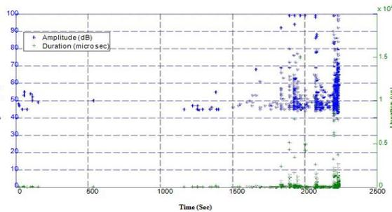
Fig.4.5.i. Time vs. Amplitude & Duration-Zero ply specimen
