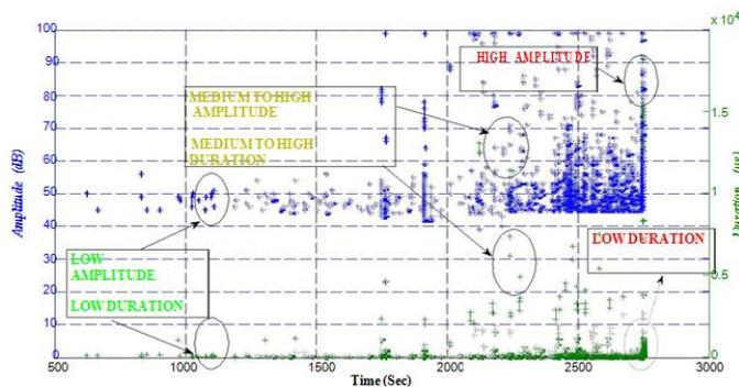
**Fig.4.5.c. Time vs. Amplitude & Duration-Cross ply specimen**
