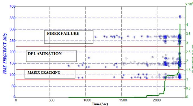
**Fig.4.5.b. Time vs. Peak frequency & cumulative counts-Zero Ply specimen**
