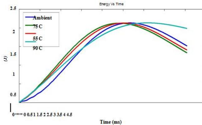
*Fig.4.3.a. Total Energy vs. time for Zero plies specimens*
