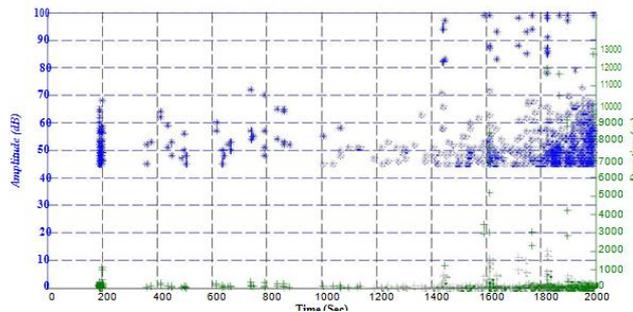
**Fig.4.5.g. Time vs. Amplitude & Duration-Cross ply specimen**
