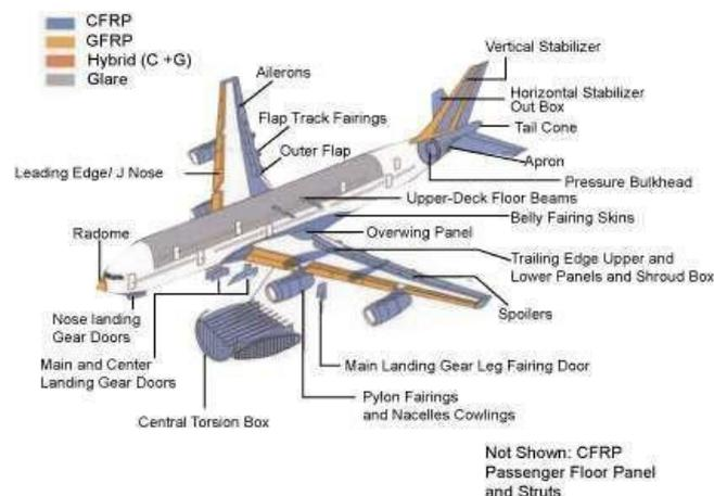
*Fig.1.b. Airbus A380 Composite Profile*
