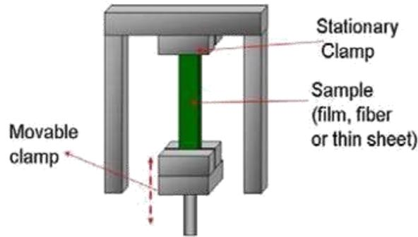
*Fig.3.e. Tension clamp for DMA*
