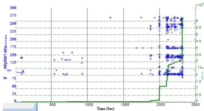
**Fig.4.5.f. Time vs. Peak frequency and cumulative counts-Zero Ply specimen**
