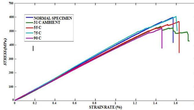
*Fig.4.4.b. Stress Vs Strain for Cross ply specimens*
