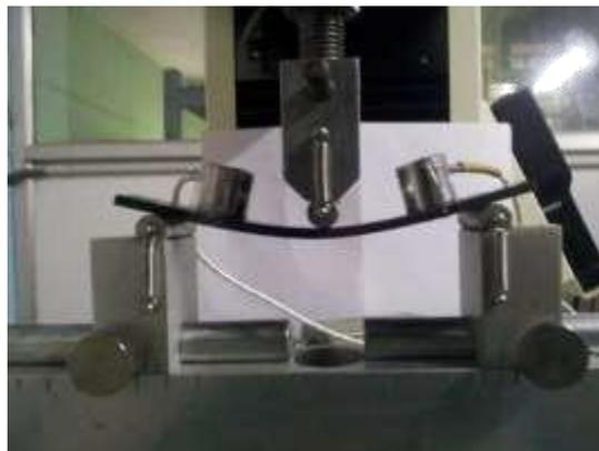
*Fig.3.j. Flexural Testing with AE Sensor position*
