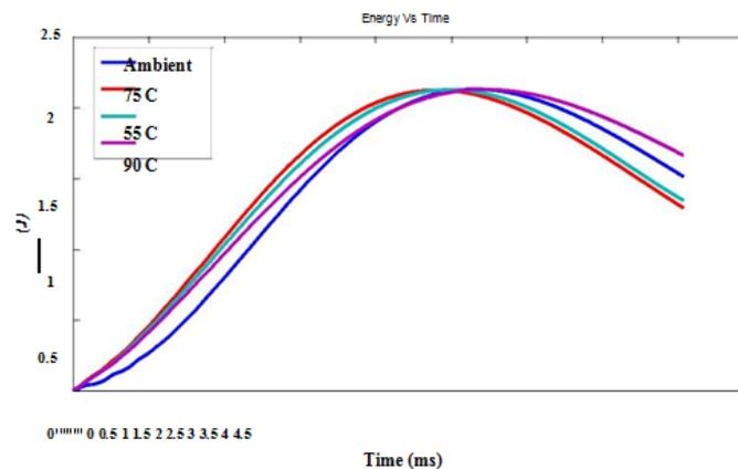
*Fig.4.3.b. Total Energy vs. time for Cross ply specimens*
