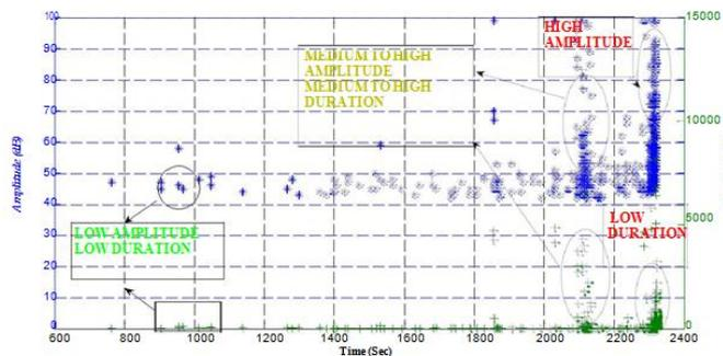
**Fig.4.5.a. Time vs. Amplitude & Duration-Zero ply specimen**
