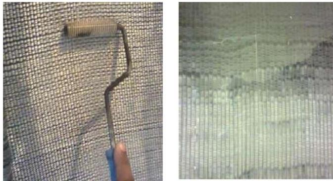
**Preparation of CFRP specimens**
