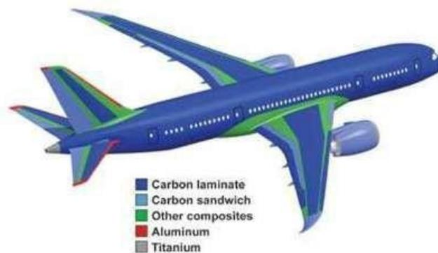
*Fig.1.a. Boeing-787 Dreamliner Composite Profile.*
