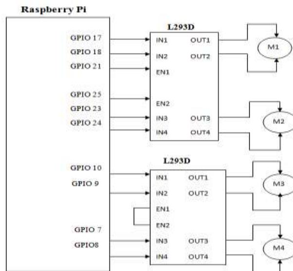
**Figure 5: Dc motor driver IC's connecting with GPiO pins of Raspberry Pi**
