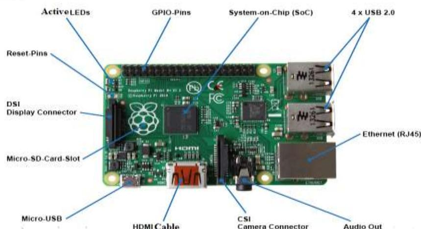
**Figure 1: Raspberry Pi Model B+**
