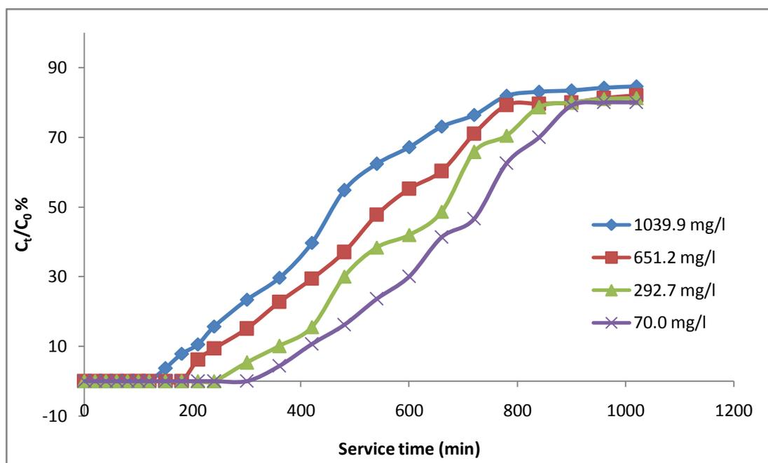
**Fig. 5. Effect of phenol concentration on breakthrough curve. . (Amount of MCFA= 10 grams, Bed Height = 13.5 cm, Influent flow rate = 1.0 ml/min, Initial concentration C<sub>0</sub> = 70.0, 292.7, 651.2 and 1039.9 mg/L)**
