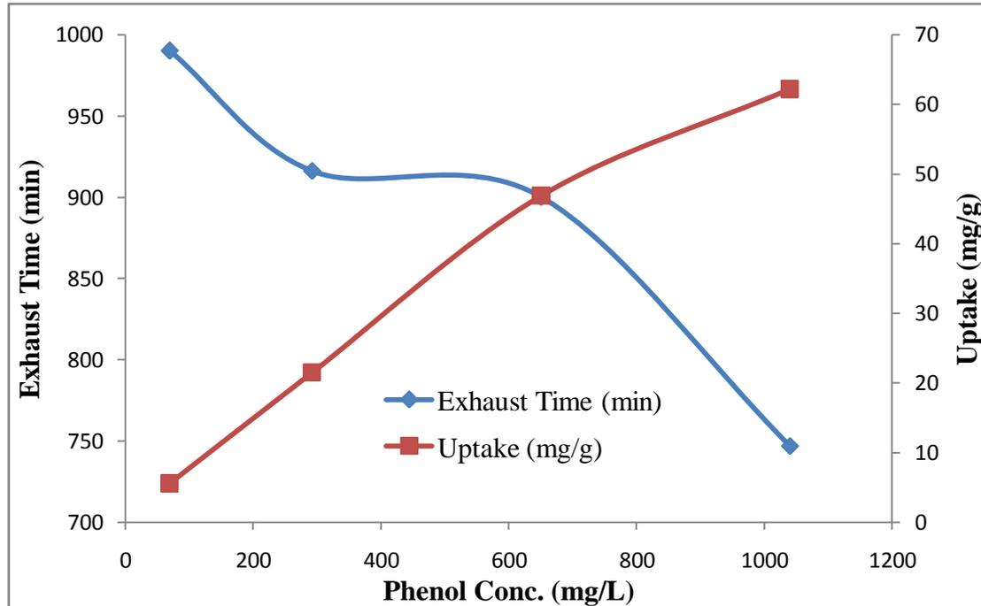
Fig. 6. Effect of phenol concentration on uptake and exhaust time. (Amount of MCFA= 10 grams, Bed Height = 13.5 cm, Influent flow rate = 1.0 ml/ min, Initial concentration  $C_0 = 70.0, 292.7, 651.2$  and  $1039.9$  mg/L)
