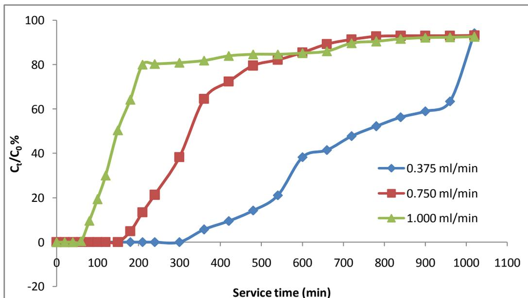
**Fig. 3. Effect of flow rate on breakthrough curve. (Conditions:- pH=6, Amount of MCFA= 10 grams, Bed Height = 13.5 cm, Initial concentration C<sub>0</sub> = 1039.9 mg/L)**
