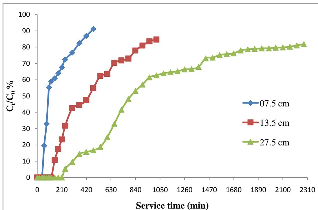
Fig. 1. Effect of bed height on breakthrough curve. (Conditions:- pH=6, Amount of MCFA= 5, 10 and 20 grams respectively, Influent flow rate = 1.0 ml/ min, Initial phenol concentration (C0) = 1039.9 mg/L)
