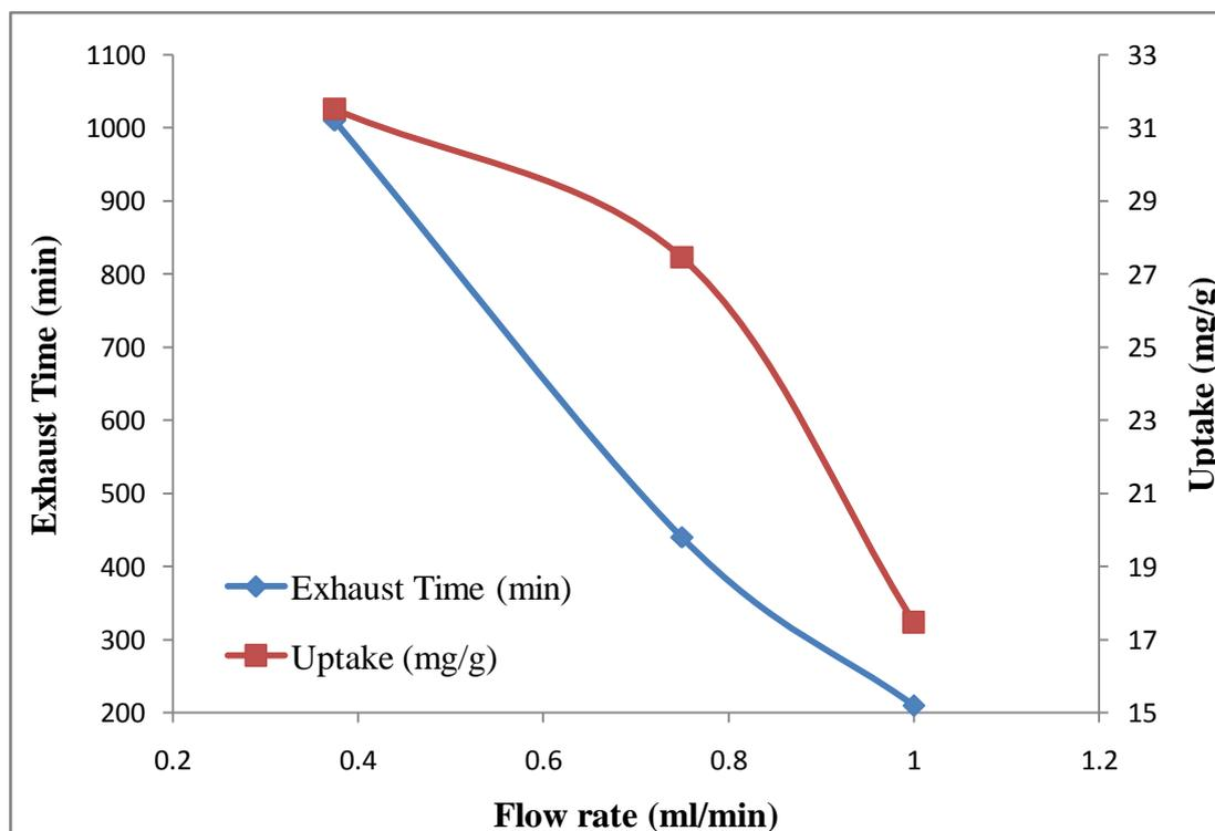
Fig. 4. Effect of flow rate on uptake and exhaust time. (Conditions:- pH=6, Amount of MCFA= 10 grams, Bed Height = 13.5 cm, Initial concentration C0 = 1039.9 mg/L)
