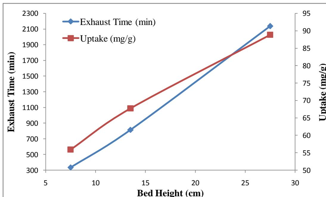
Fig. 2. Effect of bed height on uptake and exhaust time. (Conditions:- pH=6, Amount of MCFA= 5, 10 and 20 grams respectively, Influent flow rate = 1.0 ml/ min, Initial concentration (C<sub>0</sub>) = 1039.9 mg/L)
